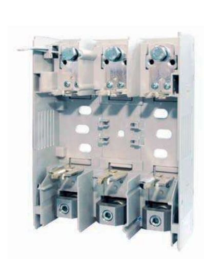
RBK 1 VD-M for installation on mounting plate, picture of fuse switch disconnecter without fuse links cover and terminal shrouds, top cable terminal - M screws, bottom cable terminal - V-clamps, (RBK 1 VG-M - bottom cable terminal - M screws, top cable terminal - V-clamps)
