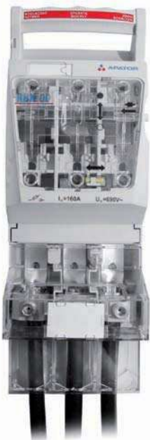
RBK 00 pro-V120 with double V-clamp for connection of two sector-shaped conductors with cross-section up to 120 mm 2 each
