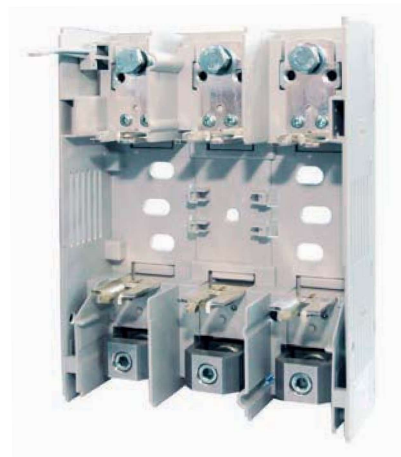
RBK 1 pro VD-M for installation on mounting plate, picture of fuse switch disconnect without fuse links cover and terminal shrouds, top cable terminal - M screws, bottom cable terminal - V-clamps, (RBK 1 pro VG-M - bottom cable terminal - M screws, top cable terminal - V-clamps)
